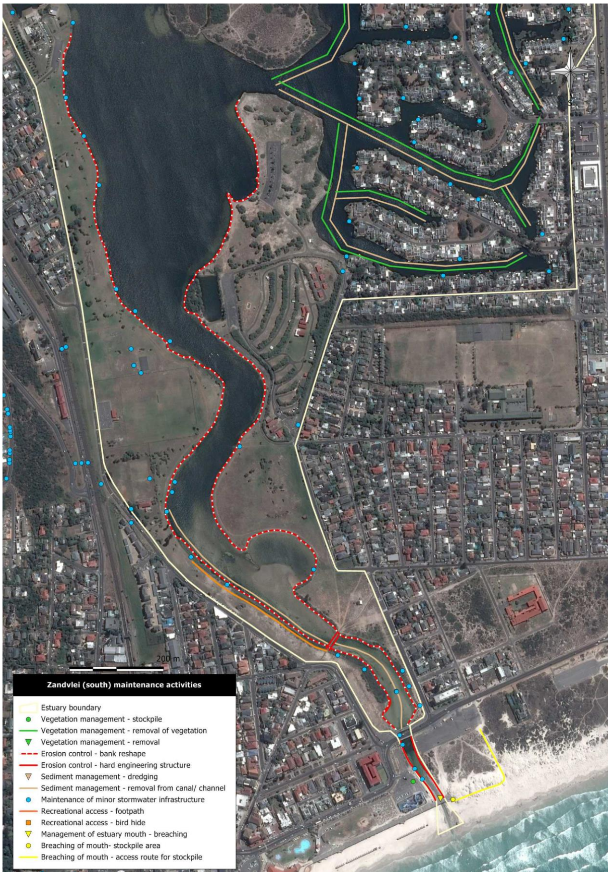
Figure 3. Location of required maintenance measures within the southern section of the Zandvlei estuary.
